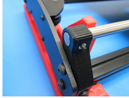
Set the Y guide rods flush to the corner, secure with set screw
