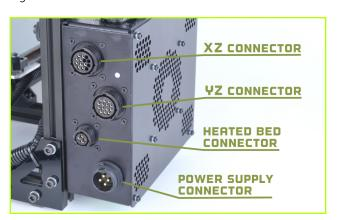
The top most connector matches the large straight plug from the XZ cable. The next connector down matches the large angled plug from the YZ cable. The third connector matches the smallest plug, from the heated bed cable.
