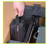
While keeping the printer in the box, pick up by the black aluminum frame and rotate the printer and foam 90 degrees - setting it upwright within the box. Make sure name plate at top is UP. Remove top foam.
