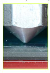
**B** To lower or raise the Z home height, adjust the Z end stop trigger, which is on the far left of the printer, mounted on the X axis motor mount. Lower it by turning clockwise and raise it by turning counter-clockwise. Once you have homed the axes and the hot end and bed have reached the correct temperature, it is time to print!
