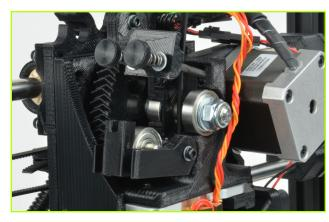
C Once the filament extrudes a small amount out of the nozzle, raise the idler and slide the two idler bolts and plate back into place. Tighten the two idler bolts. Tighten the two screws until the top of the thumbscrews are about 10mm away from the plastic clin
