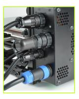
Locate the USB plug on the front of the TAZ electronics enclosure. Plug in the USB cable, square B plug end, into the USB receptacle on the front of the electronics enclosure. Plug the A end of the USB cable into your computer.
