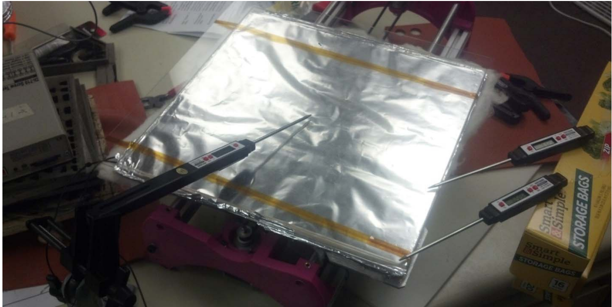
Figure 5. Pictures of Preliminary Prototype with COTS KAPTON and Insulation
